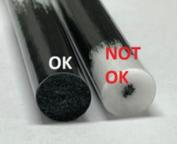
After ink injection and inserting the nib, the marker must be kept nib down for at least 1 hour.
